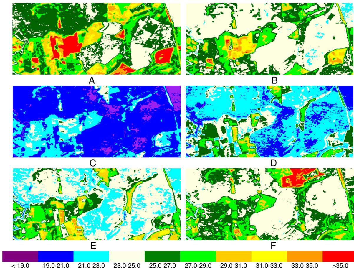
Figura 15: Cartas de temperatura ( $^{\circ}\text{C}$ ) referente os DJ 53 (A), 101 (B), 149 (C), 213 (D), 229 (E) e 325 (F).
