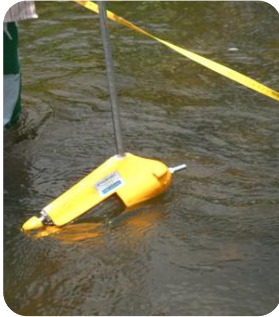
Figure 7. Suspended sediment sampling (sampler - US DH-48) in Capibaribe River.
