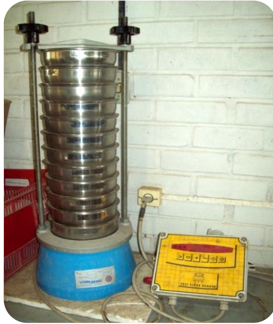
Figure 10. Test sieve shaker used to determine the particle size distribution.
