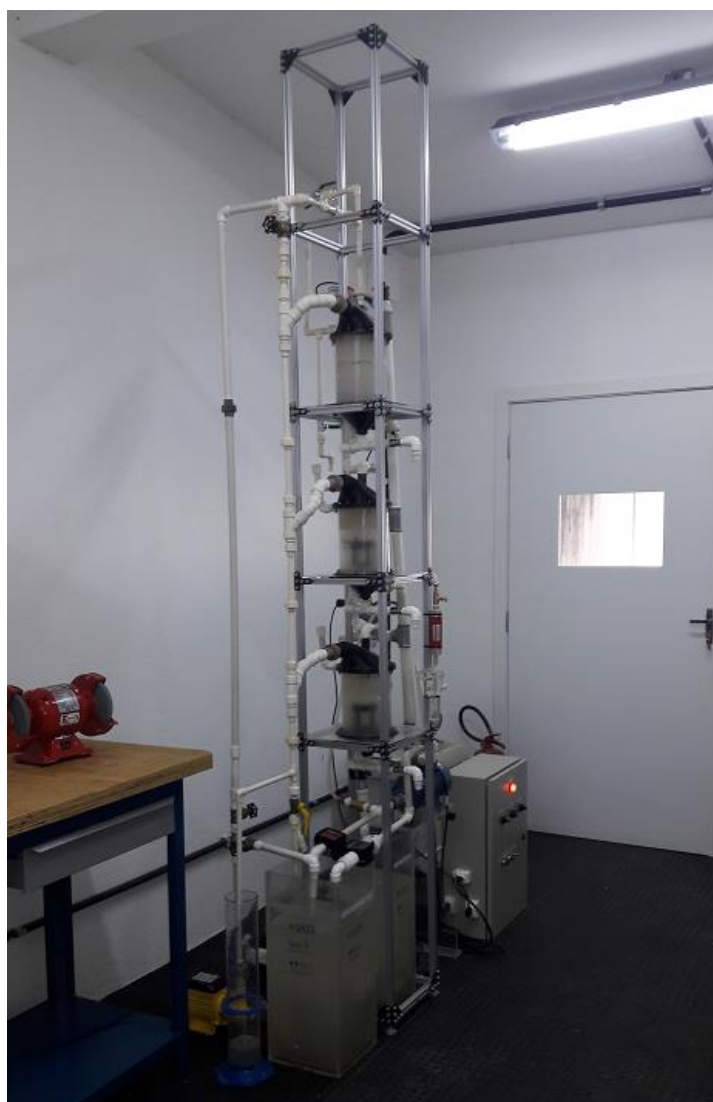
Figure 3. Bench-scale induced pre-saturation tower with different stages, author photo
