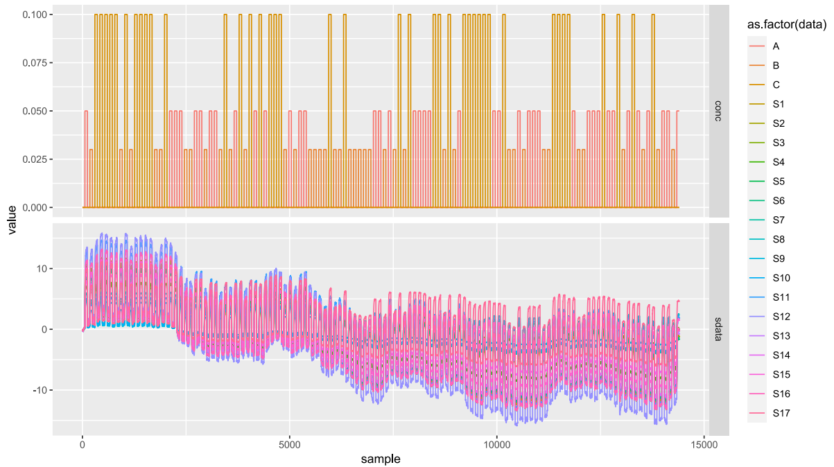
Figure 26 – Plot showing the signal responses of the sensor array when analytes at different concentrations of gases A, B, C are injected. The chronological sequence of the 360 measurements is represented in this graph. These correspond to the third work scenario (without noise and with drifts). In the upper part, the injected gases and their concentrations are represented
