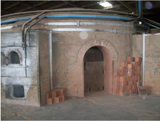
**Figura 13 – Forno contínuo (túnel)**
