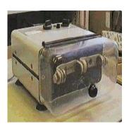
**Figure 4.** The lyophilized material is reduced to a powder using a Mechanical grinder
