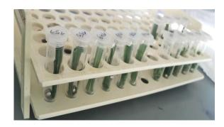
**Figure 3.** Steel beads are introduced at the bottom of each tube containing lyophilized material
